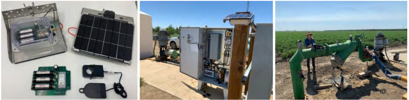
| Figure 24: Satellite connected sensors provided by Virridy and installation in Solano County project.
