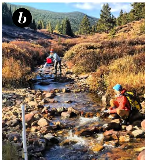
Figure 31: Examples of low-cost headwater catchment monitoring. (a) Cameras pointed at demarcated poles measure snow depth; (b) pressure transducers within PVC pipe track water depth in streams. Salt dilution stream discharge measurements are being conducted in (b).
